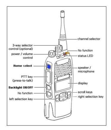
When in use the TAIT radio is always searching for the tower with the strongest signal. When it associates with a new tower it will sound three beeps to let you know service is available.
